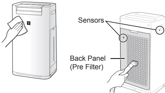
Remove the dust gently with a cleaning tool such as a vacuum cleaner.
