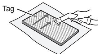
Maintain only the tagged surface. Do not clean up the opposite surface. The filter is fragile, so be careful not to apply too much pressure.
