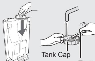
Clean the inside of the Water Tank with a soft sponge and the Tank Cap with a cotton swab or toothbrush.
