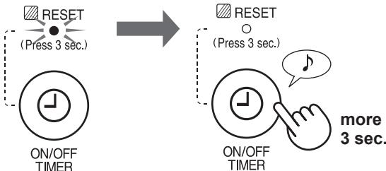
This is a reminder to perform the maintenance described below. After performing maintenance, reset the Filter Indicator.
